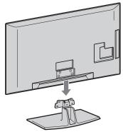
3 Fix the TV to the stand according to the arrow marks ★ that guide the screw holes using the supplied screws.
